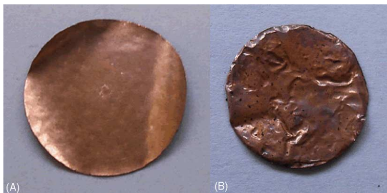
Fig. 3. Back side view of the Si:C composite electrodes. Active material pasted on a copper foil. Left image: before cycling; right image: after cycling.
